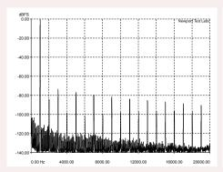
**Graph 2:** Total harmonic distortion (THD) at 1kHz at an output of 1-watt into a 4-ohmnon-inductive load, referenced to OdB. [Redgum Magnificata Power Amplifier]
