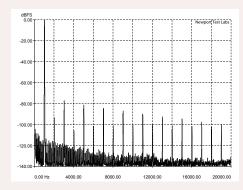
**Graph 1:** Total harmonic distortion (THD) at 1kHz at an output of 1-watt into an 8-ohm non-inductive load, referenced to 0dB. [Redgum Magnificata Power Amplifier]
