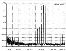
**Graph 5:** Intermodulation distortion (CCIF-IMD) using test signals at 19kHz and 20kHz, at an output of 1-watt into an 8-ohm non-inductive load, ref. to 0dB. [Redgum Magnificata]
