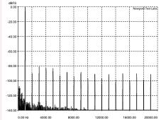
**Graph 4:** Total harmonic distortion (THD) at 1kHz at an output of 550-watts into a4-ohm non-inductive load, referenced to 0dB. [Redgum Magnificata Power Amplifier]
