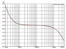
**Graph 6:** Frequency response of line input at an output of 1-watt into an 8-ohm non-inductive load (black trace) and into a combination resistive/ inductive/capacitive load representative of a typical two-way loudspeaker system (red trace). [Redgum Magnificata Power Amplifier]
