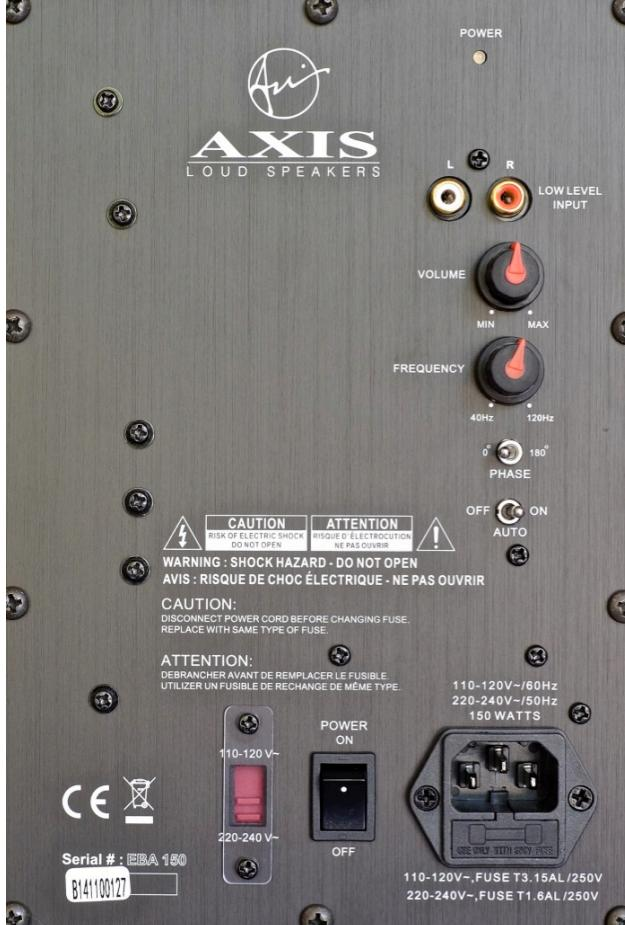
The amplifier requires AC power. Insert the supplied IEC power cable into the power socket but *do not* switch on yet. Ensure that the correct mains voltage has been set by the red slider switch to the left of the power button.
