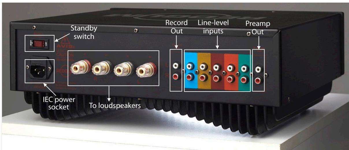
If you have a turntable ensure that the signal from its pickup cartridge is first connected to a phono pre-amp such as the REDGUM RGPH2ENR. The output of the phono pre-amp can be connected to any of the inputs on the back of your amplifier.
